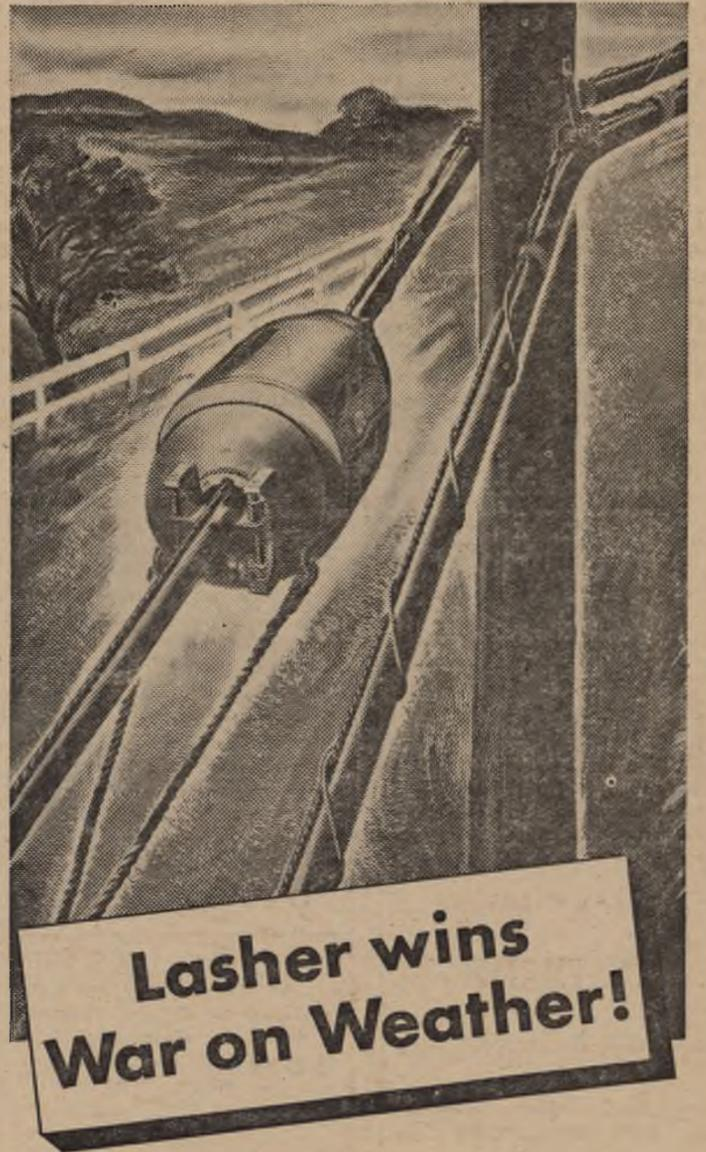
For years, telephone cable has been hung by stiff wire rings from its supporting strand. But repeated expansion and contraction caused by temperature changes sometimes proved too much for even the best cable sheath. Fatigue cracks developed near the poles—this meant leaks—possible service interruptions—expensive repairs.
