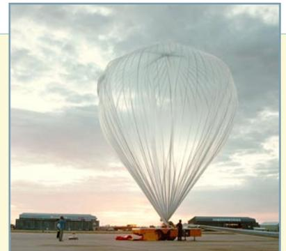
A balloon like this, thinner than a garbage bag and filled with six million cubic feet of helium, will haul the 2.5 ton BalloonWinds payload aloft to 100,000 ft. Photo courtesy of Holloman Air Force Base
